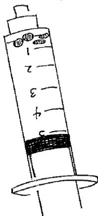
5. Put your finger over the syringe tip and pull the plunger. This will create a vacuum which will pull the air and oxygen from the leaf discs.
